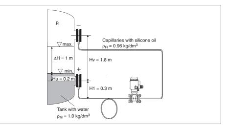
Pressure on the negative side of the differential pressure transmitter (p-) when the tank is empty (min. level)
