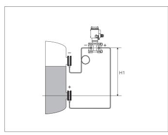
Installation above the lower diaphragm seal
