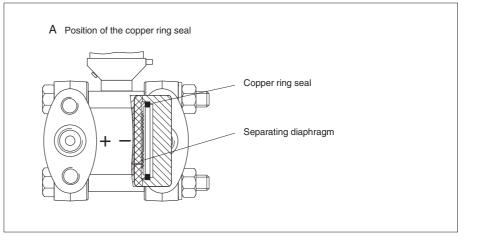
Copper ring seal for Deltabar S FMD 630, FMD 633
