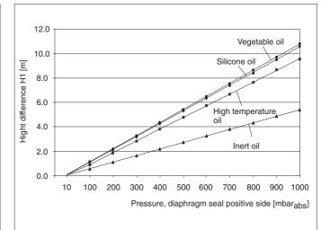
Diagram of maximum installation height above the lower diaphragm seal for vacuum applications dependent on the pressure at the diaphragm seal on the positive side.
