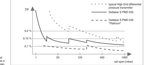
Graph showing "Total Performance" (TP) as a function of the set span.
