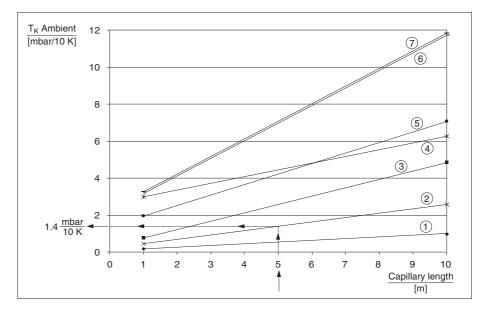
Diagram T<sub>K Ambient</sub> dependent on the capillary length for FMD 633
