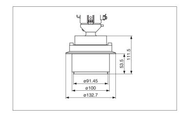
Sanitary connection with 2" extension negative side ¼ -18 NPT • Version WH: AISI 316L (1.4435)
