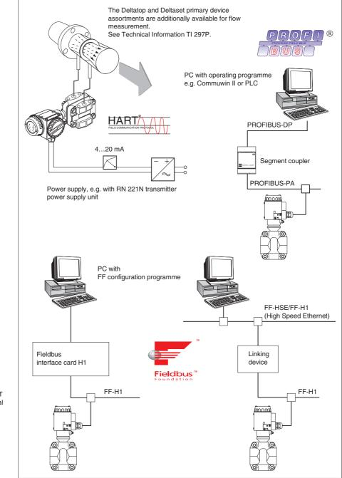
Complete measuring system Deltabar S • *left above:*
