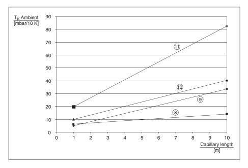
Diagram T<sub>K Ambient</sub> dependent on the capillary length for FMD 633
