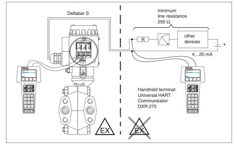
The HART Communicator DXR 275 can be connected anywhere along the 4...20 mA line.
