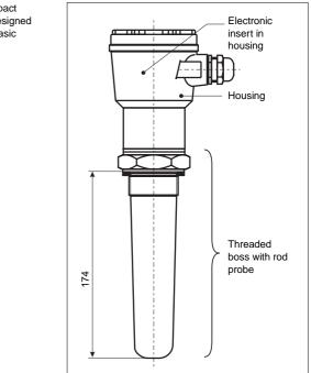
The Nivocompact FTC 731 is designed using these basic modules.
