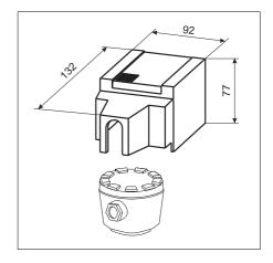
Dimensions of protective sun cover (accessory). This cover prevents condensation in the housing.
