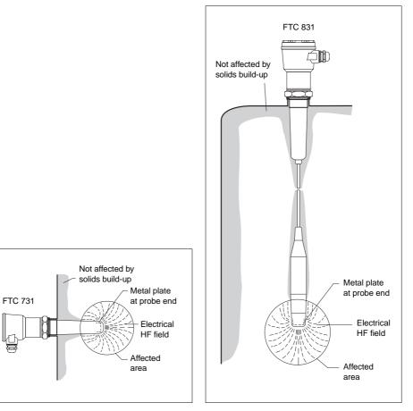
The operation of the Nivocompact FTC 831 with rope probe is totally unaffected by material build-up on the walls of the silo.
