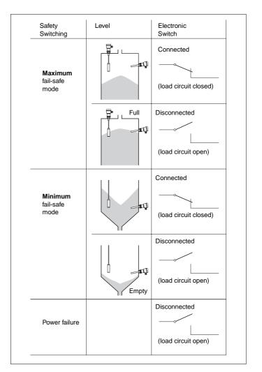
The electronic switch operates according to the fail-safe switching and the level.
