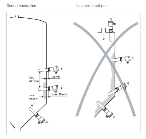
a) The probe tip points slightly downwards so that material can slide off more easily;
