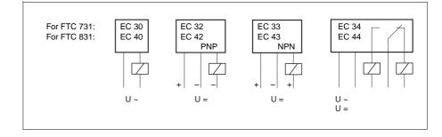
Electrical connections available with the different electronic inserts.
